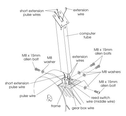
Figure 7 - Install Computer Tube
